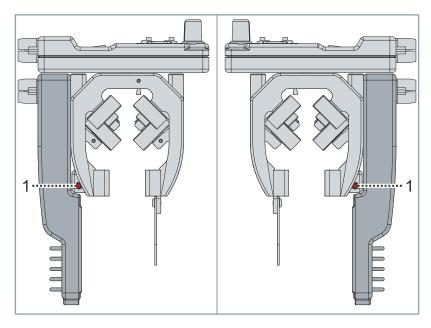
On both sides of the mover there is a set screw [1] for adjusting the position of the NCT electronics. The air gap between the NCT electronics and the module can be adjusted using the two set screws.
