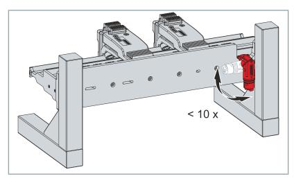
The connector of the module may be rotated by 90° a maximum of ten times.
