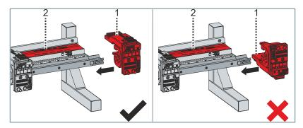
The NCT electronics [1] must be located on the side of the name plate [2] when the mover is inserted.
