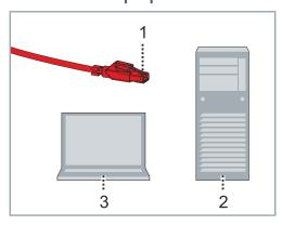
▶ Plug the connector [1] of the data line into the corresponding port of your PC [2] or laptop [3]
