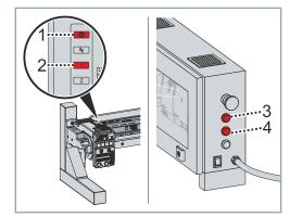
The *Power* LED [1] on the NCT electronics light up continuously. The LED 1 [2] on the NCT electronics must flash continuously. The *Start* button [3] on the control cabinet must flash green. The *Stop* button [4] on the control cabinet must go out.
