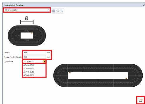
The small preview image shows the shape of the selected XTS system. The large display shows the exact system size and module arrangement for the set parameters.
