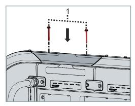
➤ Tighten screws with sealing rings 1 hand tight to fix the rail on support
