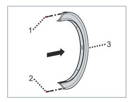
▶ Insert locating pins 1 and 2 into the curved rail 3
