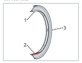
► Grease the support surfaces 1 and 2 of the curved rail 3 with Vaseline
