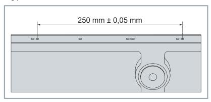
The distance between the center of the first locating pin bore for one module to the center of the first locating pin bore for the next module must be 250 mm. The manufacturing tolerance is  $\pm$  0.05 mm.
