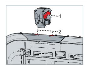
▶ Make sure when mounting the movers that the guide rollers 1 of the movers do not press against the edges 2 of the rail on support
