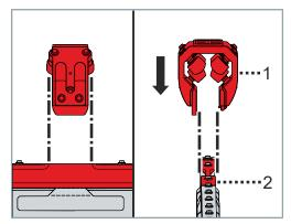
► Place mover 1 carefully with both hands centrally onto the rail on support 2
