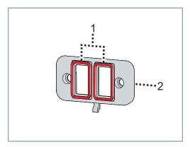
► Grease all O-ring contours 1 of the seal 2 for the electrical interface with Vaseline
