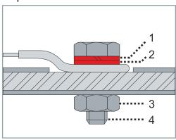
► Earth unpainted surface as shown in the figure with spring washer 1, washer 2, nut 3 and bolt 4
