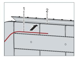
► Press seal 1 into the groove 2 on the other side of the system in the same way
