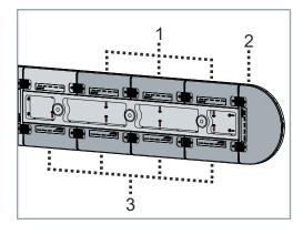
▶ Place further modules 1, the second curved module 2 and further modules on the opposite side 3 in a row, thereby screwing in screws with sealing rings, leaving only a minimal gap in each
