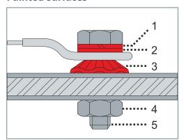
► Earth painted surface as shown in the figure with spring washer 1, washer 2, contact washer 3, nut 4 and bolt 5
