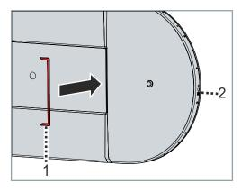
► Mount the short end of seal 1 on the other side of the curved module 2 in the same way
