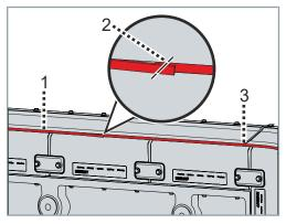
► Cut diagonally through both ends 2 of the overlapping seals 1 and 3 with a cutting tool
