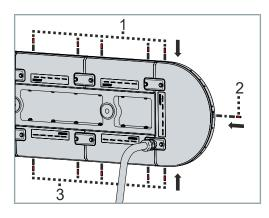
► Insert locating pins 1, 2 and 3 in all straight modules and both curved modules
