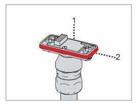
Grease the edge 2 on the cover with power supply 1 with Vaseline
