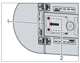
Screw in the screws 2 of the curved module hand tight in order to fix the seals 1 on both sides
