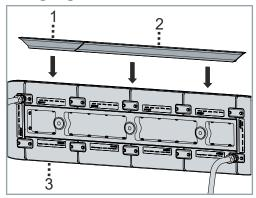
► Always use guide rail 2 with lock 1 at the top on the assembled system 3
