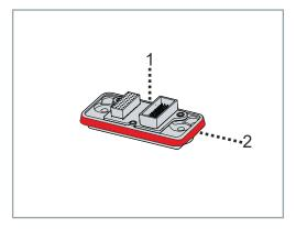
► Grease the edge 2 on the cover with connection card 1 with Vaseline
