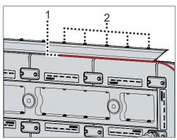
Screw in the screws 2 of the guide rail hand tight in order to fix the seals 1 on both sides of the system
