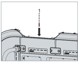
▶ Push guard plate 1 over the set screw onto the module
