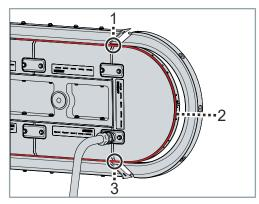
► Grease seals 2 between guide rail and curved rail 1 and 3 on both sides of the system with Vaseline
