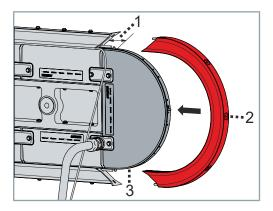
► Push curved rail 2 onto the curved module 3 up to a distance 1 of approx. 30 mm
