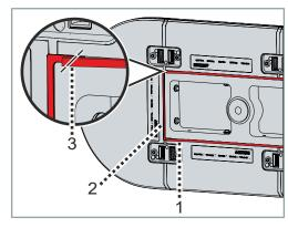
► Cut diagonally through both ends 3 of the overlapping seals 1 and 2 with a cutting tool
