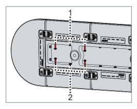
➤ Screw in all screws with sealing rings 1 and 2 on the two remaining modules hand tight
