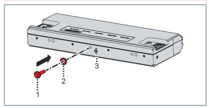
When screwing the screw with seal 1 into the tapped hole with the marking "functional earth" 3, use a contact washer 2 between the machine bed and the seal.
