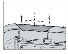
► Screw set screw 1 into the module
