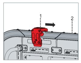
► Carefully push the mover 1 by hand along the guide rail 2 and out of the rail on support
