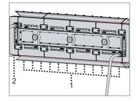
➤ Screw in the screws 1 of the guide rail hand tight in order to fix the seals 2 on both sides of the system
