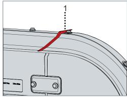
► Cut off the overhanging part of the seal 1 flush to the rail with a cutting tool
