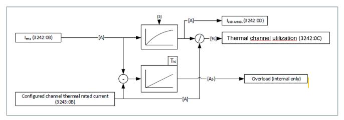
Initially, the AX8000 monitors and limits the actual current to the "configured channel peak current". If the "Thermal Channel Utilization" increases to a value of >100%, the limitation is reduced to the "configured channel rated current". If the Thermal Channel Utilization drops below 100%, the limit is raised again to the "configured channel peak current".
