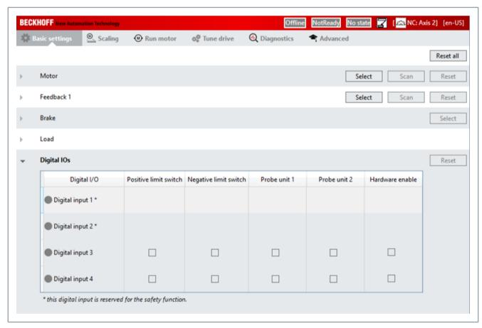
The activation of the functions is done by checking the appropriate box. In the following picture, for example, a positive limit switch and a touch probe. The logic of the switch can be changed by selecting the buttons below the tick. (break contact / make contact)
