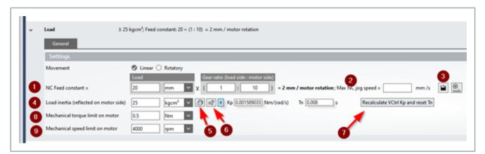
"Load inertia (reflected on motor side)" [4], represents the mass inertia acting on the motor shaft. The value is included in the control and improves the axis behavior. "Calculate Load Inertia Manually" [5] supports you in calculating the effective mass inertia. Via the button "Identify load inertia automatically. Go to "tune drive - Advanced Tuning" for details." [6] will take you to the Advanced Tuning function.
