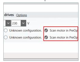
Motors of the AM8000 and AM8500 series with electronic type plate are automatically scanned and transferred to the configuration.
