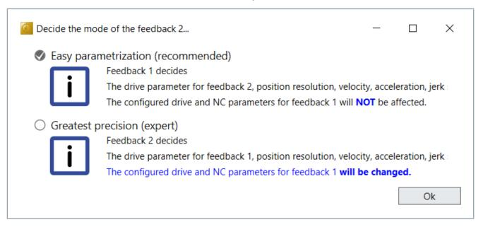
Easy parametization (recommended): the scaling of the second feedback is referred to the first feedback. Settings from the NC are not changed.
