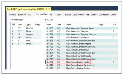
► Select "0x1A32 ChA Torque Control Inputs"
