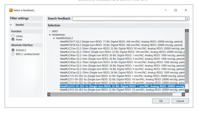
In the next step, a dialog box opens to specify the scaling of the second feedback system.
