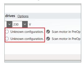
If you select this option, your axis module is transferred into the configuration with its default values. You can change the basic settings later in the project.
