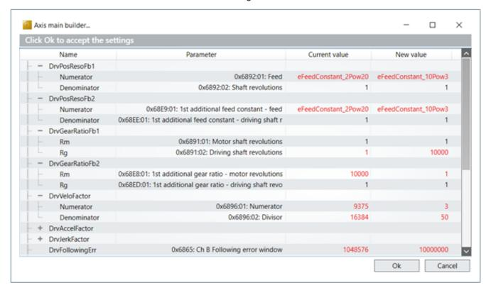
If the Greatest precision mode was selected during commissioning, the necessary changes in the NC must be applied by clicking on Save NC parameters.
