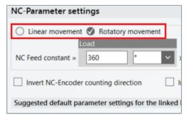
In the selection area for "NC parameter settings" you can size your mechanical system and thus determine the "NC Feed constant".
