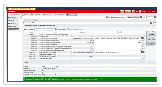
As soon as the command has finished, the results are displayed at the bottom of the DM2. In the above case, the motor could move freely (mandatory for the command), the sense of rotation of the encoder matches the sense of rotation of the rotating field in the stator and an absolute offset of 239.95° was determined.
