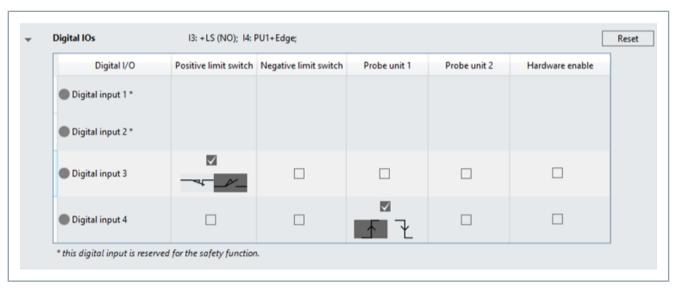
If you use an input as hardware enable you have the choice between the reaction "Torque off" or "Closed Loop Ramp".
