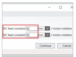
This function defines the distance travelled per motor revolution. Adjust the mechanics via the "Scaling" menu.
