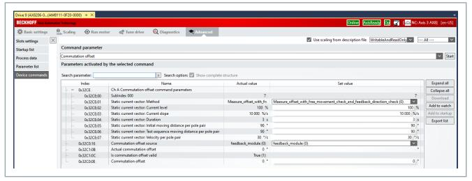
▶ Double-click on the channel of an AX8000 for which the commutation angle is to be determined.
