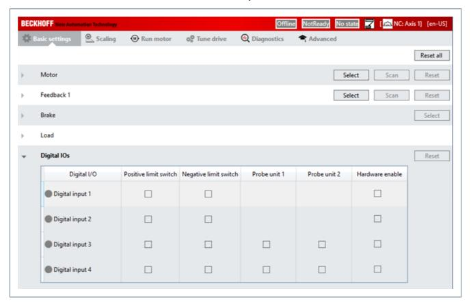
AX8xxx-x2xx device with Safety / Digital input 1 and 2 are preassigned Safety inputs
