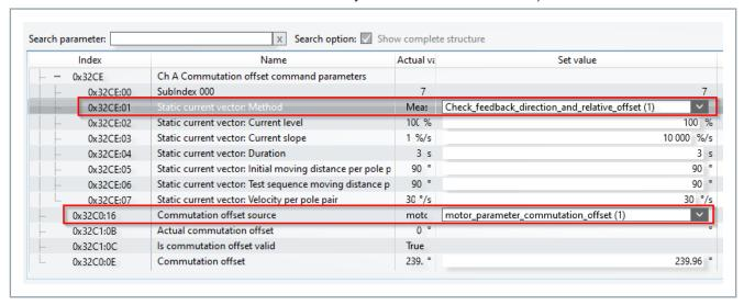
The setting "Check\_Feedback\_direction\_and\_realative\_offset (1)" determines the commutation offset relative to the currently parameterized offset.
