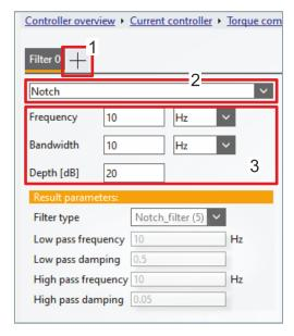
A new filter is inserted by left-clicking on the plus symbol [1]. The available options [2] are:
