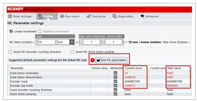
Activate the configuration and check whether the two feedback systems have the same counting direction.
