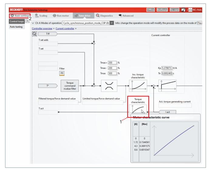
The curve for third-party motors is parameterized on the "Basic settings" tab [3] when the external motor is created.
