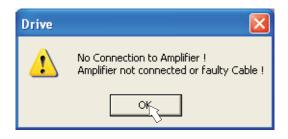
The software tries to communicate with the drive and to upload the parameters. If it's not successful, you receive this error message.
