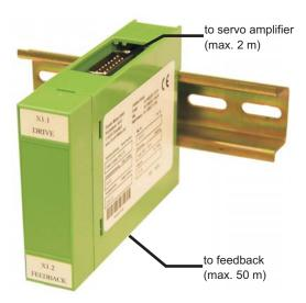
The extended power supply enables the operation of encoder systems at connector X1 with a power consumption of up to 400 mA DC. This power supply is switched between X1 and the encoder and supplied by AX 2000.
