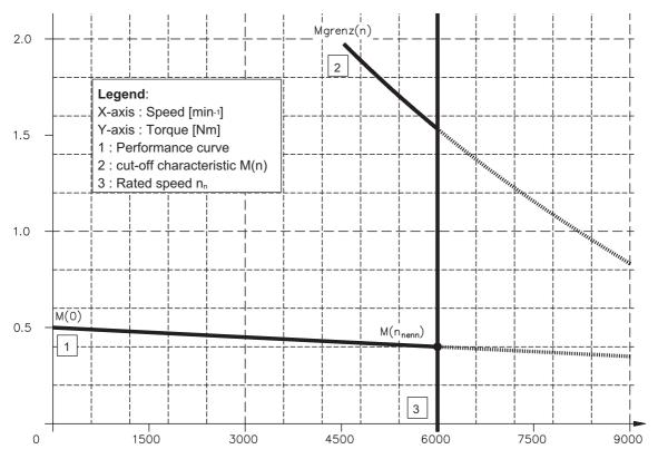
III.9 Torque characteristics AM237M
