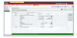
▶ Determine direction of rotation and commutation angle in parameter P-0-0166 (see also AX5000 System Manual, chapter 9.6.2)
