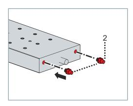
► Screw the threaded push-in fittings [2] into the holes provided
