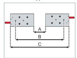
This illustration shows an example of an arrangement of two coil parts with cables laid in opposite directions.
