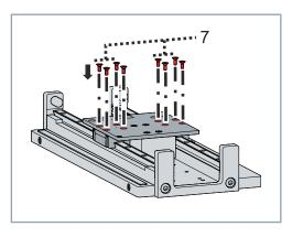
► Insert and tighten the screws [7]
