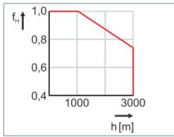
Derating may be necessary at high ambient temperature or when operating at a great height above sea level. Continuous forces are affected by the reduction.
