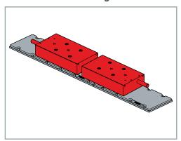
With this type of coupling, the coil parts are arranged one after the other on a common magnetic track. This type of coupling tends to be used for applications with long strokes, since a second magnetic track with associated costs is avoided.
