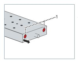
► Remove the plug [1] at the front on the coil part
