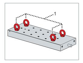
➤ Screw eyebolts [1] into the outer adjacent threads on the outer sides. Make sure to always choose the largest possible distance from each other
