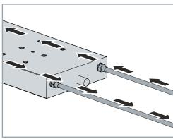
• AL806x-1: Water flow as cooling circuit
