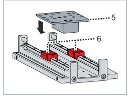
▶ Place the assembled coil part including the machine carriage [5] on the guide carriage [6]
