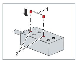
▶ Insert locating pins [1] into the holes of the coil part [2]:
