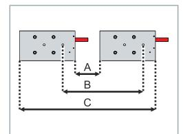
This illustration shows an example of an arrangement of two coil parts with cables in the same direction.
