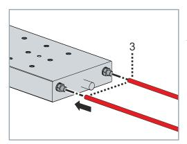
▶ Insert the cooling hoses [3] into the threaded push-in fittings
