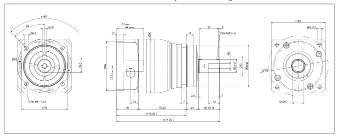
• Clamping hub diameter up to E = 19 mm
