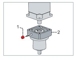
Turn the clamping hub [1] until the screw [2] can be seen above the mounting hole ► Loosen the screw [2] by one turn
