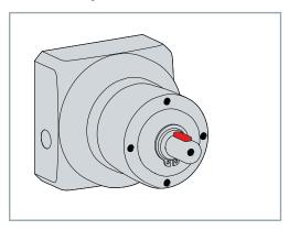
A feather key transmits torque to an output element.
