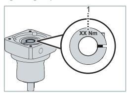
The value for the tightening torque [1] of the clamping screw is punched into the clamping hub from above.
