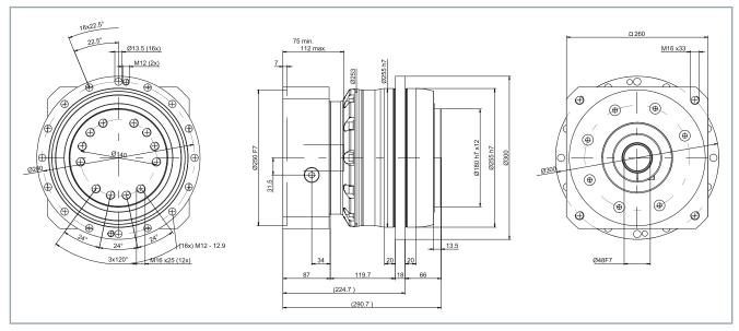
• Clamping hub diameter up to M = 48 mm
