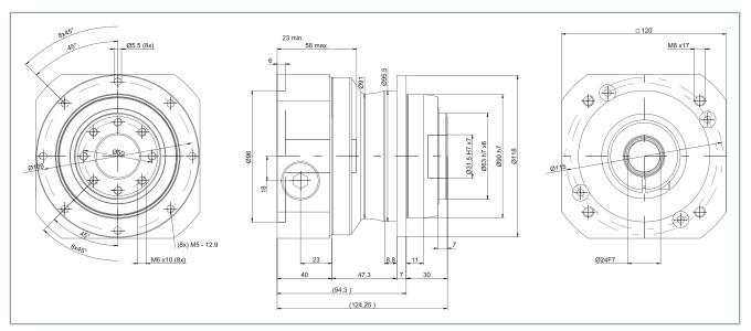
• Clamping hub diameter up to G = 24 mm
