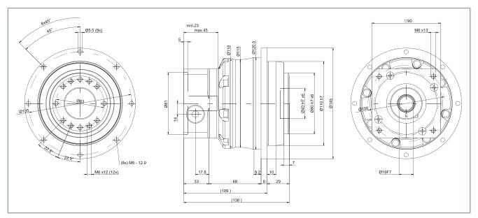
• Clamping hub diameter up to E = 19 mm
