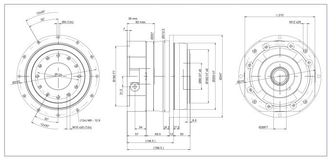
• Clamping hub diameter up to K = 38 mm
