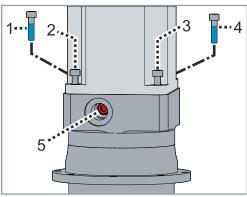
This example shows a motor size with four fixing points in the flange.
