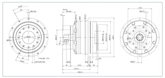
• Clamping hub diameter up to G = 24 mm
