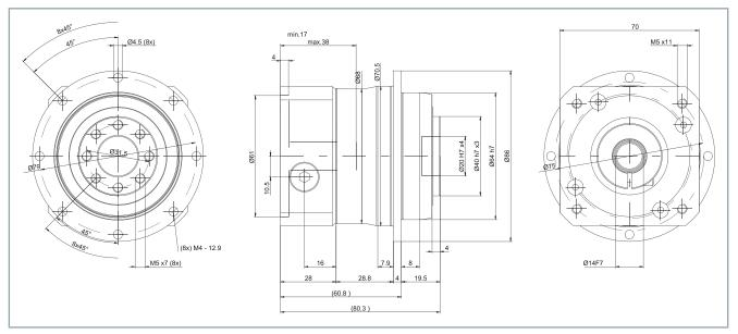
• Clamping hub diameter up to C = 14 mm
