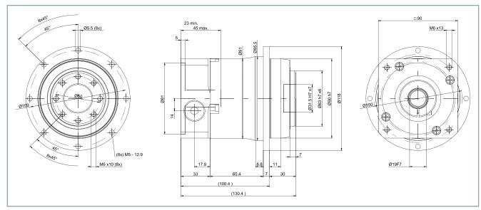
• Clamping hub diameter up to E = 19 mm
