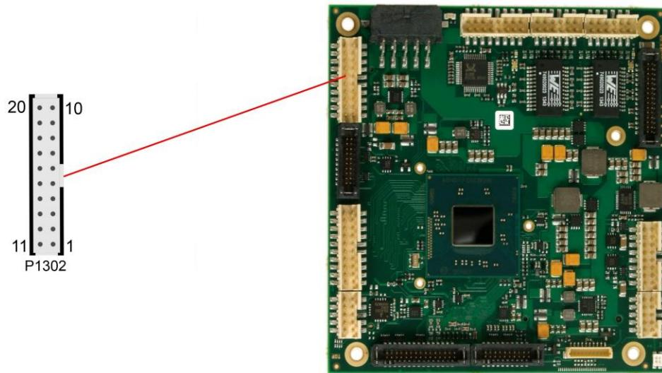
Pinout 2x10 system connector:
