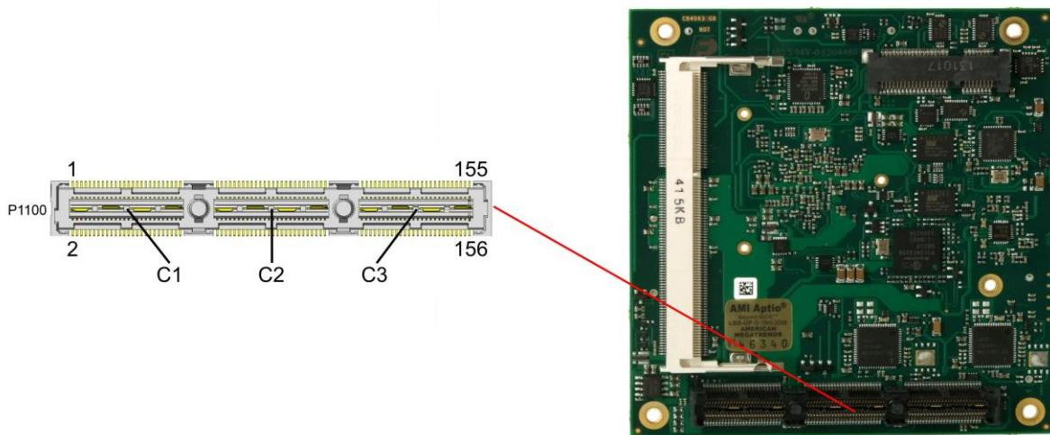
Pinout PCI104-Express connector (type 2):
