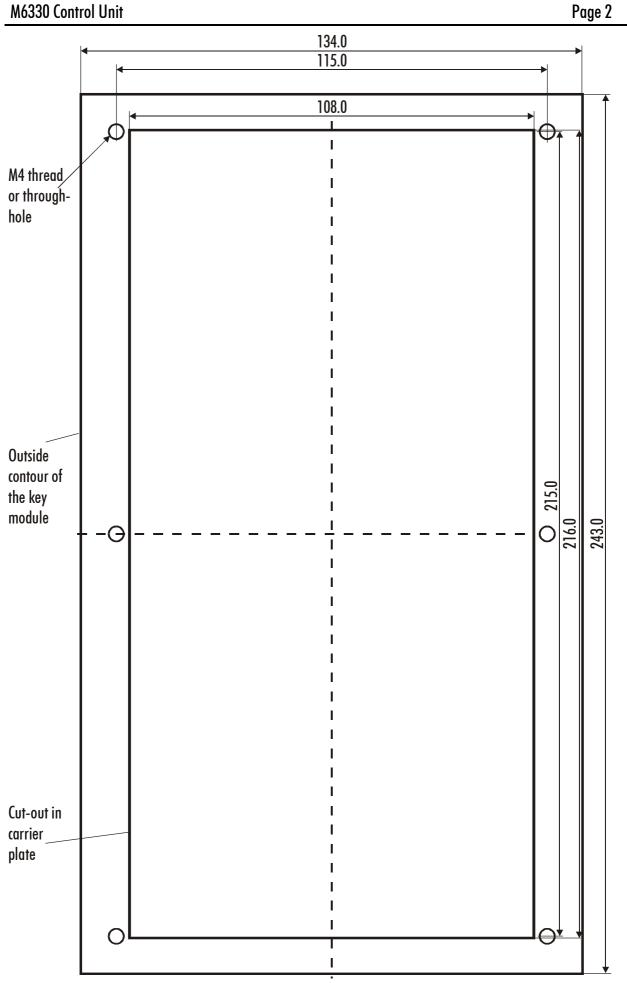
Assembly hole for the M6331 built-in panel
