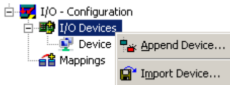
Fig. 50: Creating a new device
