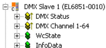
Fig. 131: TwinCAT tree DMX slave, process image up to 64 bytes of user data
