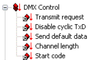
Fig. 128: TwinCAT tree DMX status, output process data
