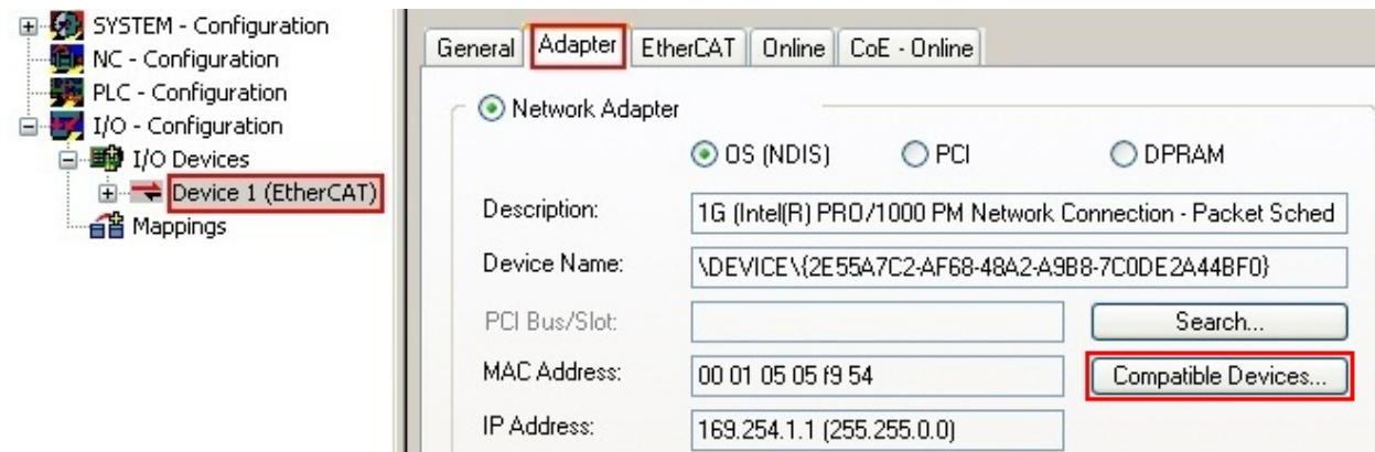
Fig. 79: EtherCAT device properties (TwinCAT 2): click on “Compatible Devices...” of tab “Adapter”
