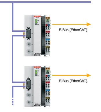
Fig. 14: PROFIBUS topology with the EK3100 Bus Coupler.
