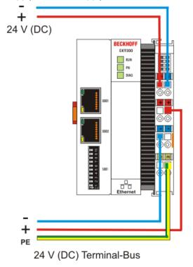
Fig. 11: Bus Coupler power supply, based on the EK9300 as an example.
