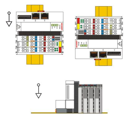
Fig. 10: Other installation positions, based on the EK9300 as an example.
