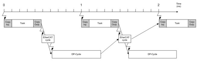
Fig. 24: Cycle with IO not at task start
