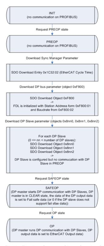
Fig. 127: Flow chart: Sequence of the configuration of the EL6731 with start SDOs
