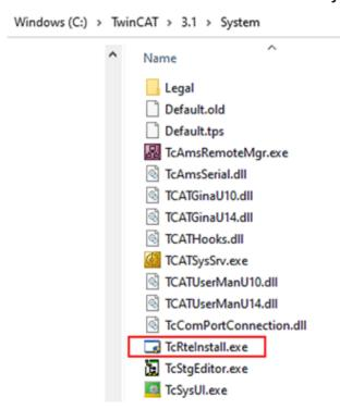
Fig. 30: TcRteInstall in the TwinCAT directory
