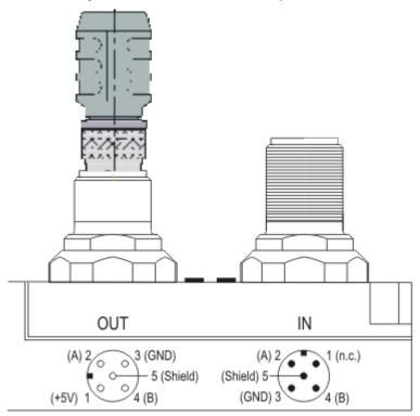
Fig. 14: Pin assignment socket/plug connector Fieldbus Box modules
