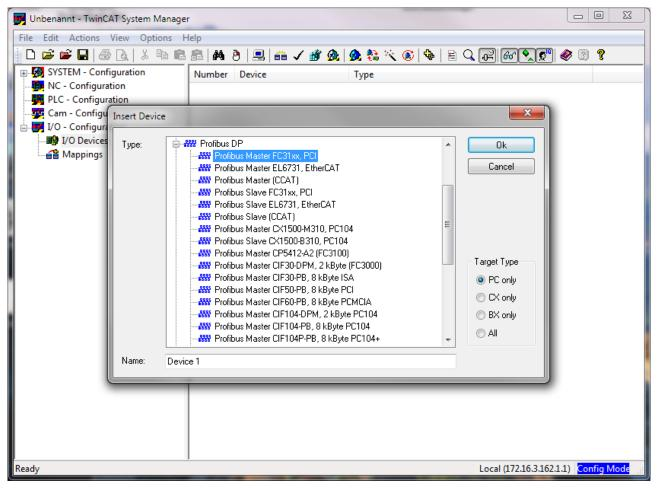
Fig. 98: Inserting an FC31xx PCI I/O device
