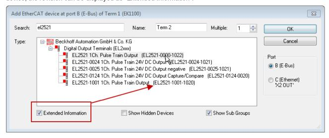
Fig. 49: Display of device revision
