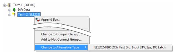
Fig. 73: TwinCAT 2 Dialog Change to Alternative Type
