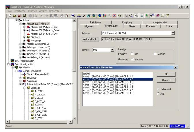
Fig. 108: Configuration, linking of axes
