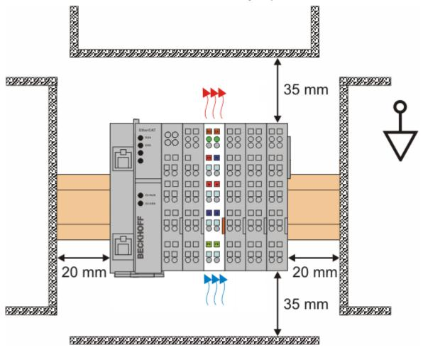
Fig. 6: Recommended distances for standard installation position
