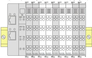
Fig. 8: Correct positioning
