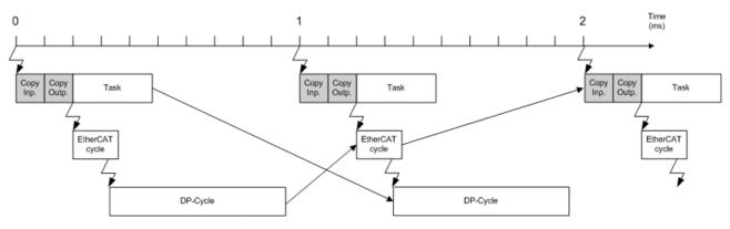
Fig. 23: Cycle with IO at task start
