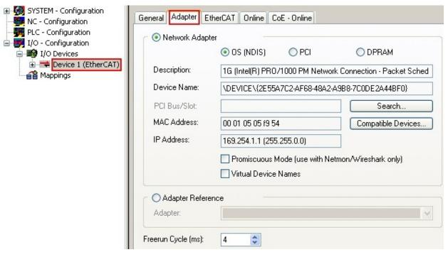
Fig. 46: EtherCAT device properties (TwinCAT 2)
