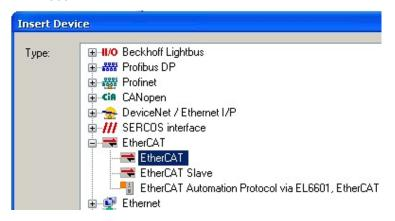
Fig. 44: Selecting the EtherCAT connection (TwinCAT 2.11, TwinCAT 3)
