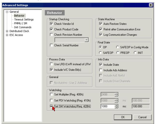
Fig. 15: eEtherCAT tab -> Advanced Settings -> Behavior -> Watchdog
