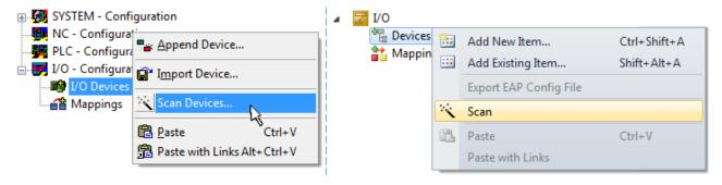
Fig. 54: Scan Devices (left: TwinCAT 2; right: TwinCAT 3)
