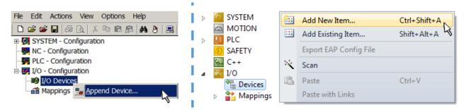
Fig. 43: Append EtherCAT device (left: TwinCAT 2; right: TwinCAT 3)
