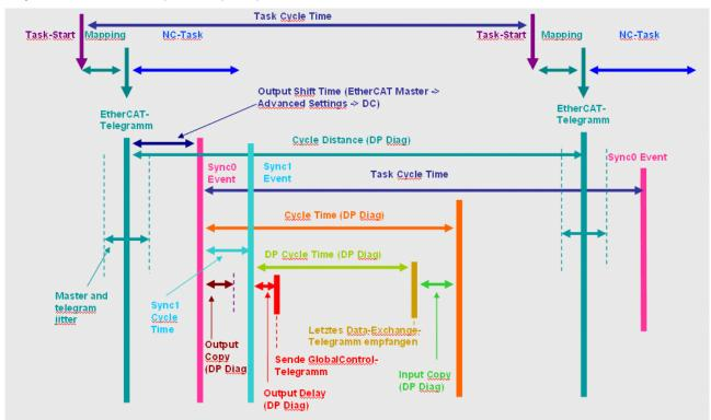
Fig. 133: DP cycle start via SYNC0, first telegram is sent after the SYNC1 event
