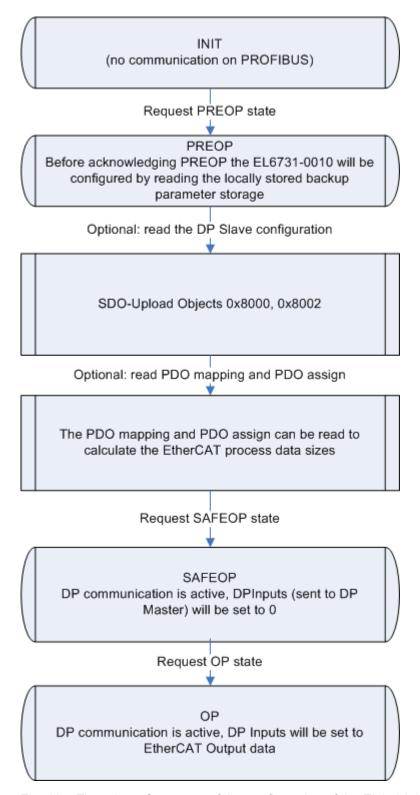
Fig. 135: Flow chart: Sequence of the configuration of the EL6731-0010 with backup parameter storage
