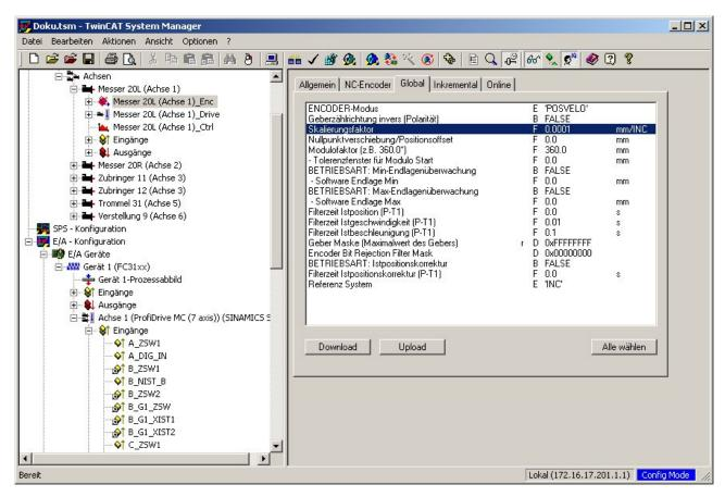
Fig. 110: "Global" tab, scaling factor entry
