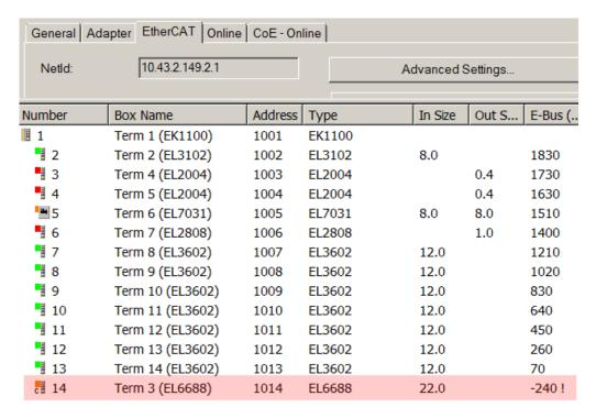
Fig. 82: Illegally exceeding the E-Bus current
