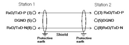
Fig. 10: PROFIBUS cable assignment
