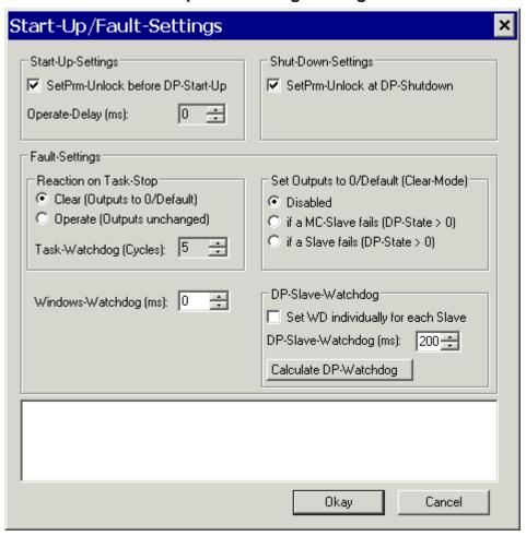
Fig. 86: Startup/fault settings dialog
