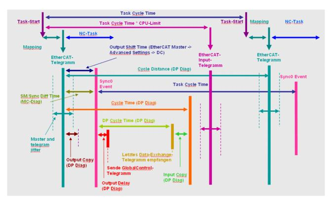
Fig. 131: Transfer of output data with LWR, input data with LRD telegram (Separate Input Update = TRUE, Task Cycle Time = Base Time)
