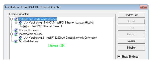
Fig. 34: Exemplary correct driver setting for the Ethernet port
