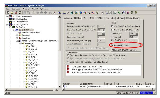
Fig. 106: MC tab, determine PB - DP cycle
