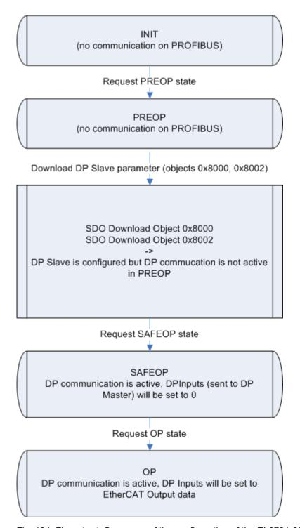
Fig. 134: Flow chart: Sequence of the configuration of the EL6731-0010 with start SDOs
