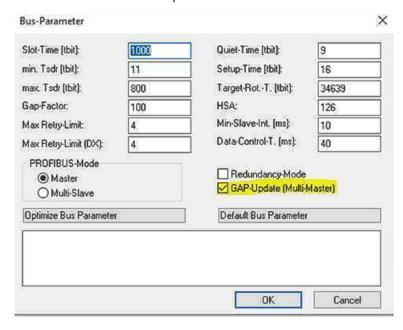
Fig. 27: Activate multi-master operation
