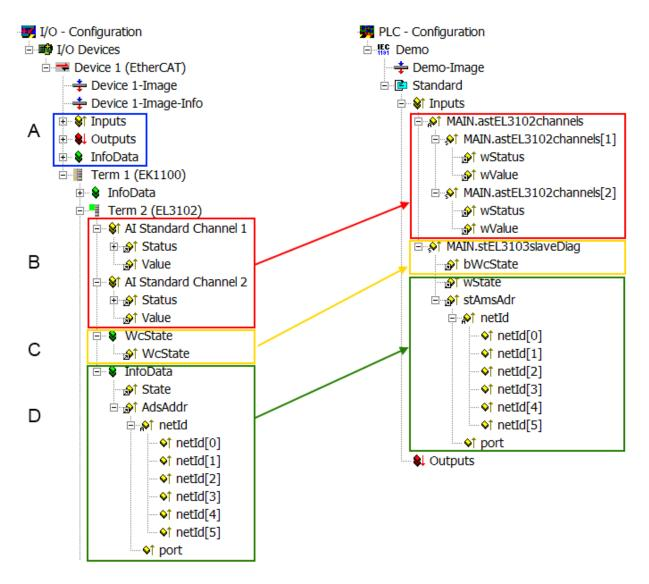
Fig. 76: Basic EtherCAT Slave Diagnosis in the PLC
