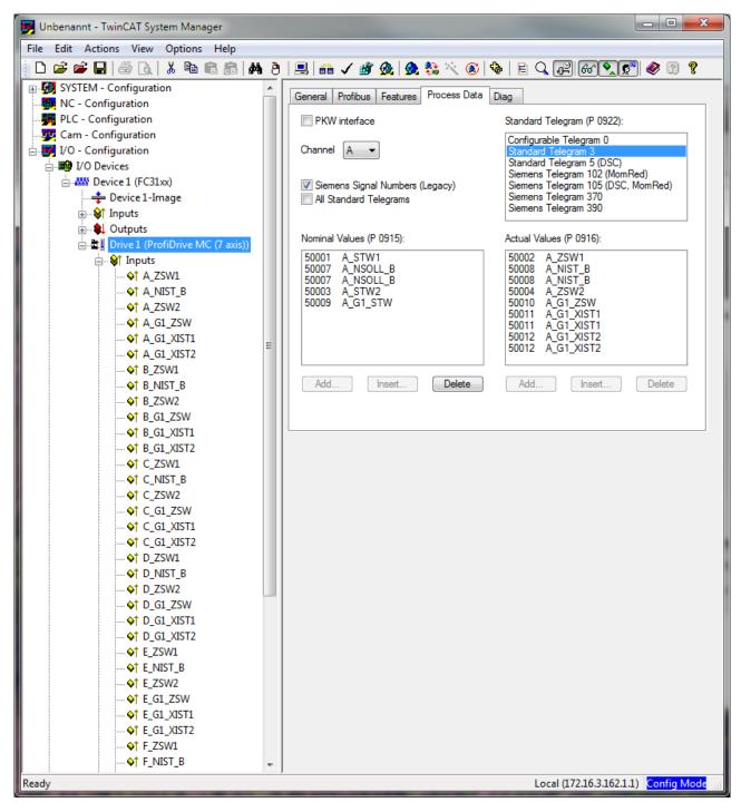
Fig. 104: Process Data tab, telegram assignment
