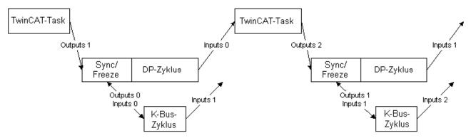
Fig. 25: TwinCAT task, DP cycle and K-bus cycle sequence
