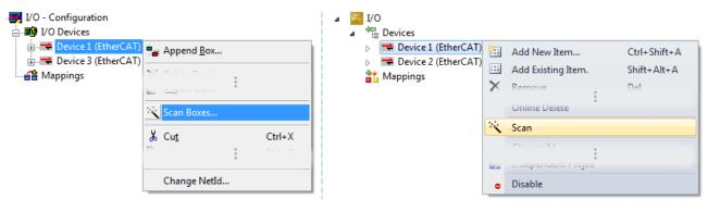
Fig. 61: Manual scanning for devices on a specified EtherCAT device (left: TwinCAT 2; right: TwinCAT 3)
