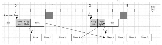
Fig. 119: Diagram showing allocation of DP slaves to several DP cycles
