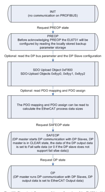
Fig. 128: Flow chart: Sequence of the configuration of the EL6731 with backup parameter storage
