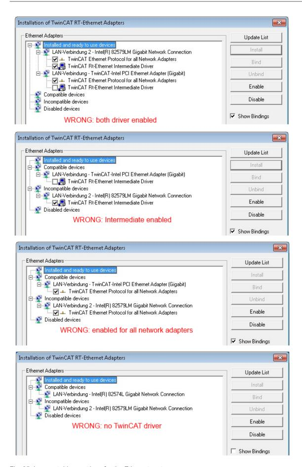
Fig. 35: Incorrect driver settings for the Ethernet port
