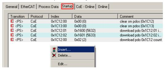
Fig. 18: Startup list in the TwinCAT System Manager
