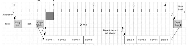
Fig. 121: Diagram showing several data samples within one task cycle
