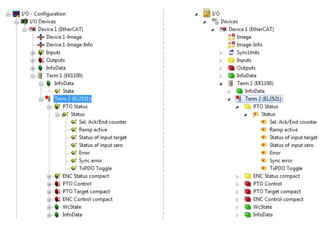
Fig. 52: EtherCAT terminal in the TwinCAT tree (left: TwinCAT 2; right: TwinCAT 3)
