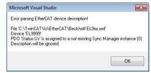
Fig. 42: Information window for faulty ESI file (left: TwinCAT 2; right: TwinCAT 3)
