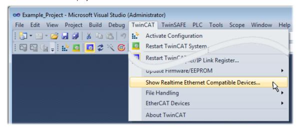
Fig. 29: Call up under VS Shell (TwinCAT 3)
