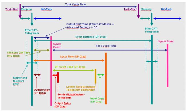
Fig. 130: DP cycle with distributed clocks and control via SM and SYNC0 event
