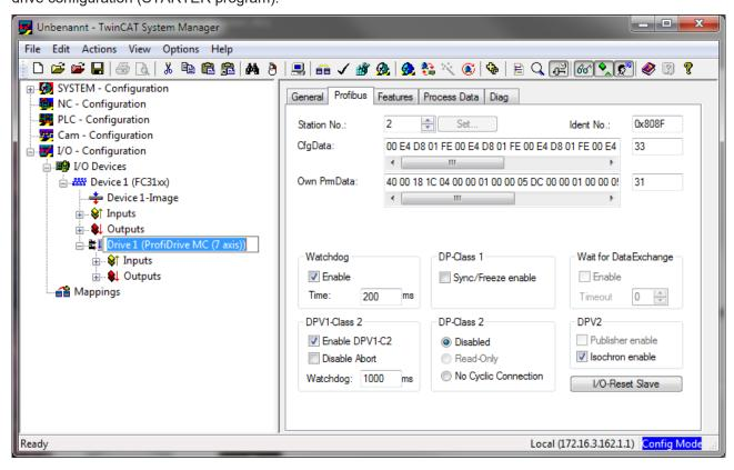
Fig. 103: Profibus tab, address selection
