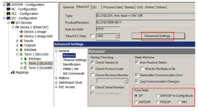
Fig. 80: Default target state in the Slave
