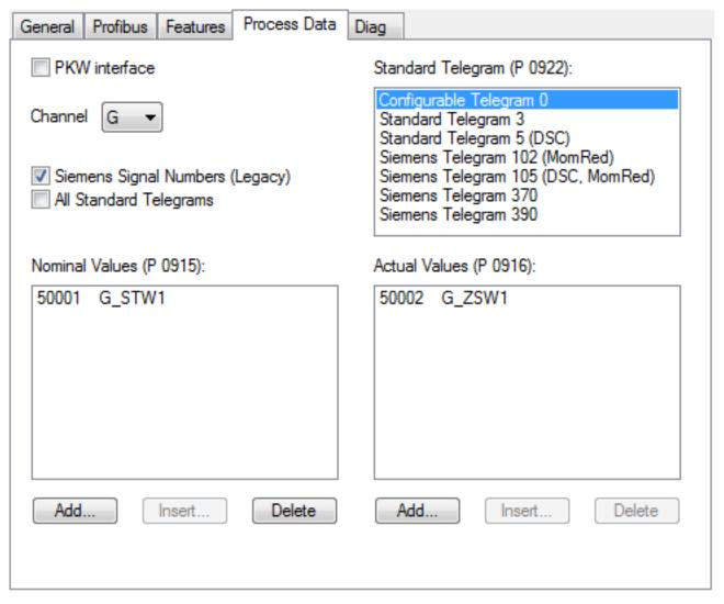
Fig. 105: Process Data tab, determine telegram
