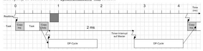
Fig. 120: Diagram showing several DP cycles in a task cycle
