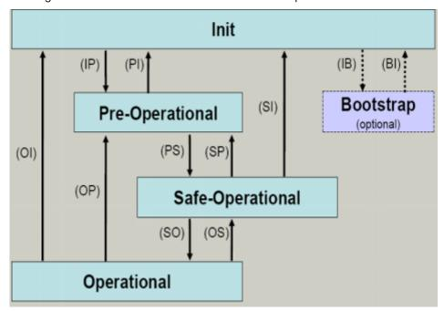
Fig. 16: States of the EtherCAT State Machine
