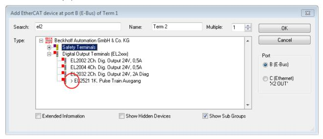
Fig. 41: Indication of an online recorded ESI of EL2521 as an example
