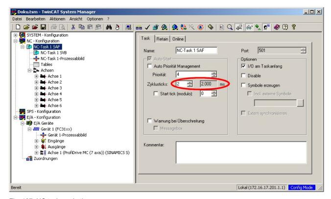
Fig. 107: NC task, cycle time
