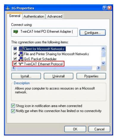
Fig. 33: Windows properties of the network interface
