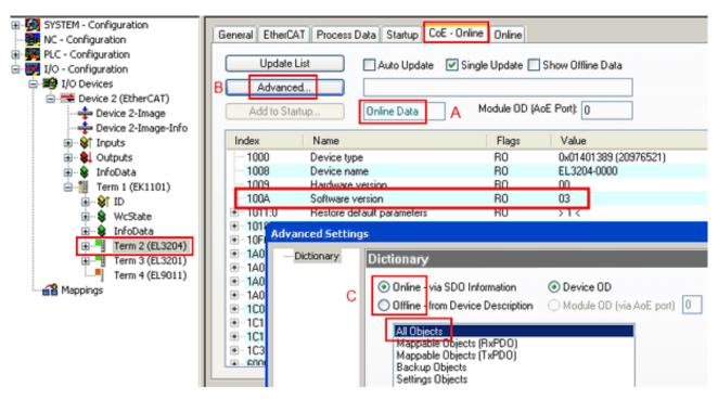
Fig. 142: Display of EL3204 firmware version
