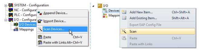
Fig. 93: Scan Devices (left: TwinCAT 2; right: TwinCAT 3)
