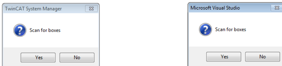
Fig. 126: Scan query after automatic creation of an EtherCAT device (left: TwinCAT 2; right: TwinCAT 3)
