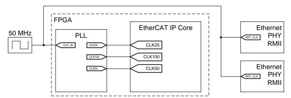
Figure 21: EtherCAT IP Core clock source (RMII)
