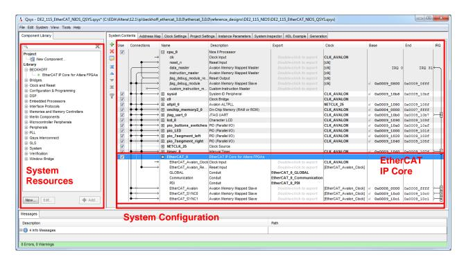
Figure 6: Qsys with EtherCAT IP Core
