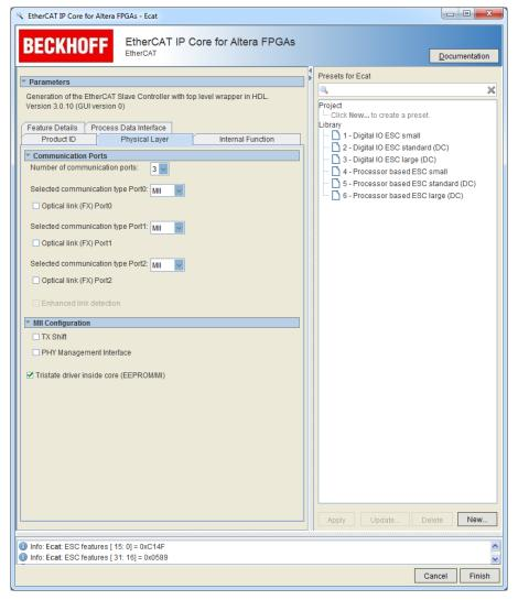
Figure 10: Physical Layer tab
