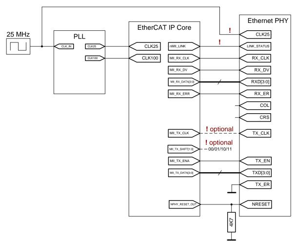
Figure 28: MII example schematic
