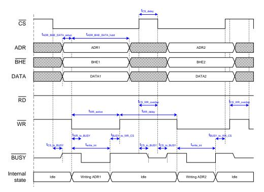
Figure 52: Write access (write after falling edge nWR)
