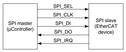
Figure 40: SPI master and slave interconnection
