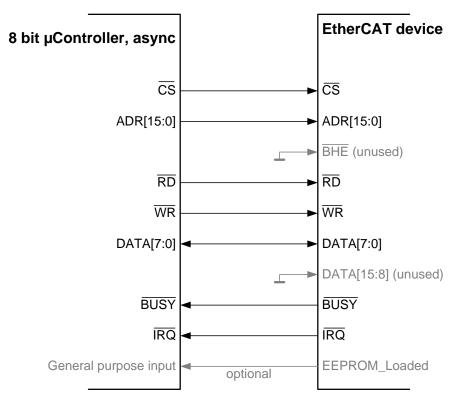
Figure 48: Connection with 8 bit µControllers (BHE and DATA[15:8] should not be left open)
