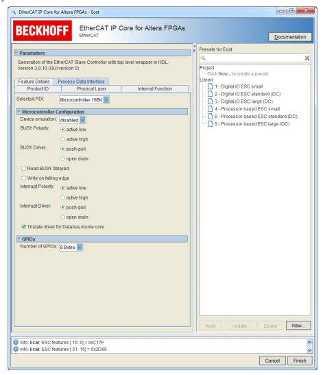
Figure 16: Register PDI – μC-Configuration
