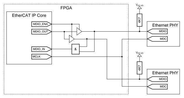
Figure 24: Example schematic with two individual MII management interfaces
