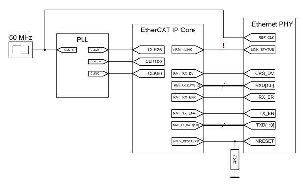
Figure 30: RMII example schematic
