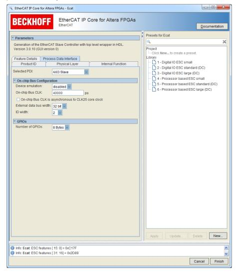
Figure 19: Register PDI - AXI3 Interface Configuration
