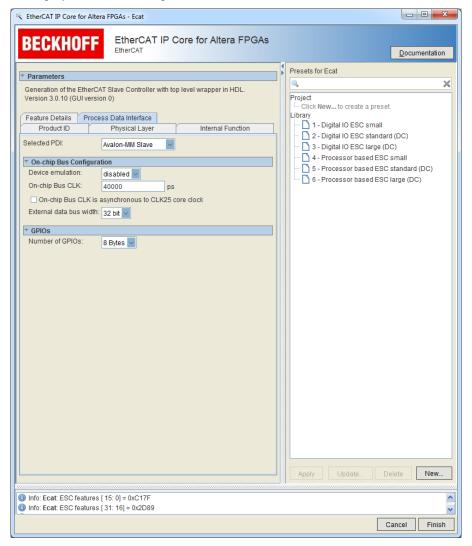
Figure 18: Register PDI – Avalon Interface Configuration
