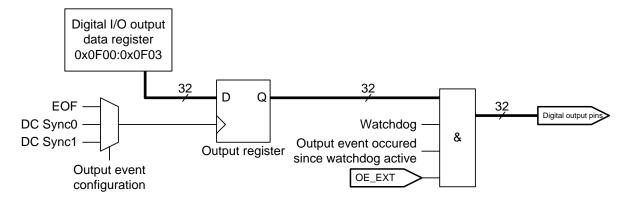
Figure 34: Digital Output Principle Schematic
