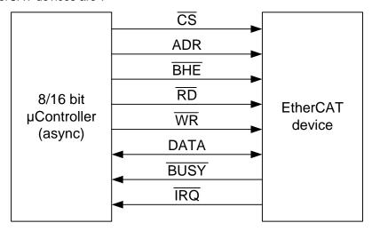
Figure 46: µController interconnection<sup>7</sup>
