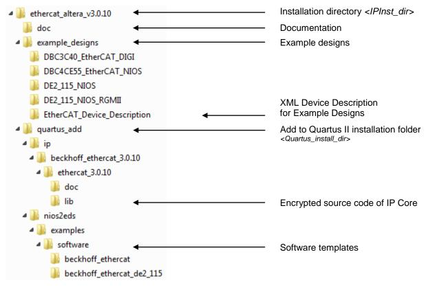
Figure 4: Files installed with EtherCAT IP Core setup
