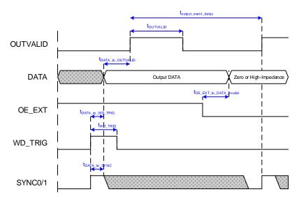
Figure 38: Digital Output timing
