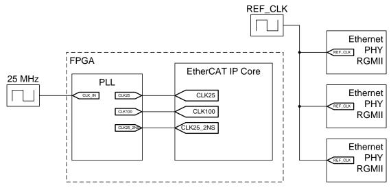
Figure 22: EtherCAT IP Core clock source (RGMII)
