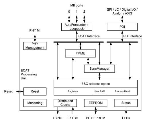
Figure 1: EtherCAT IP Core Block Diagram
