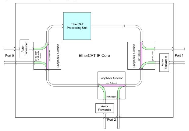
Figure 2: Frame Processing
