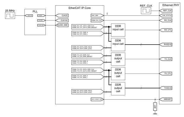
Figure 32: RGMII example schematic
