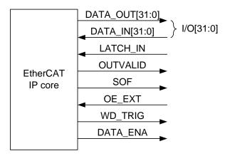
Figure 33: IP core digital I/O signals
