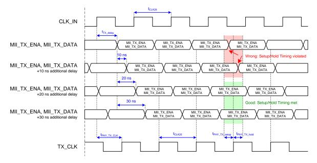
Figure 26: MII TX Timing Diagram
