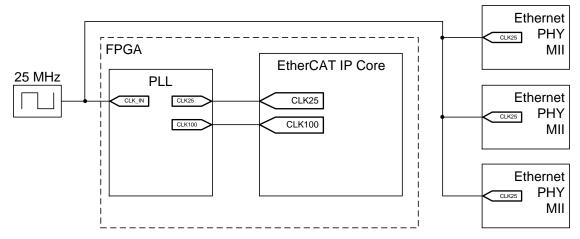
Figure 20: EtherCAT IP Core clock source (MII)
