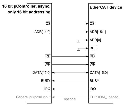
Figure 47: Connection with 16 bit µControllers without byte addressing
