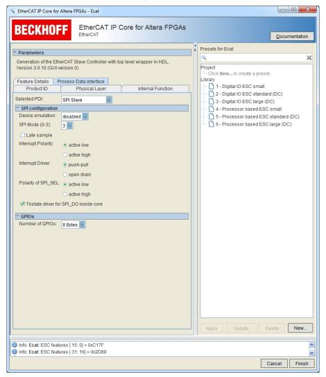
Figure 17: Register PDI - SPI Configuration
