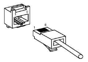
Figure 14: RJ45 Connector
