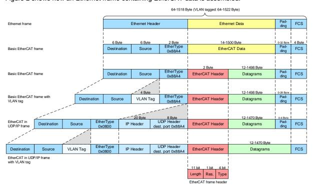
Figure 2: Ethernet Frame with EtherCAT Data
