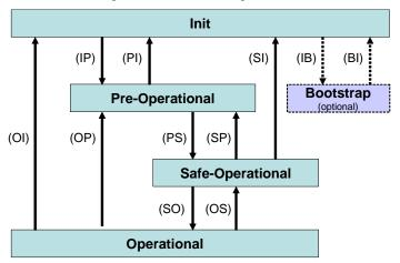
Figure 37: EtherCAT State Machine
