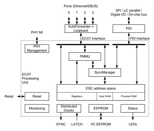
Figure 1: EtherCAT Slave Controller Block Diagram
