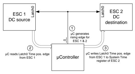
Figure 34: System Time PDI Controlled with three steps
