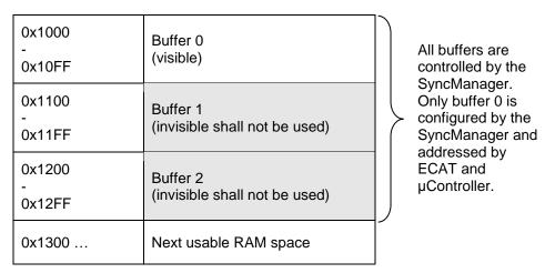
Figure 24: SyncManager Buffer allocation
