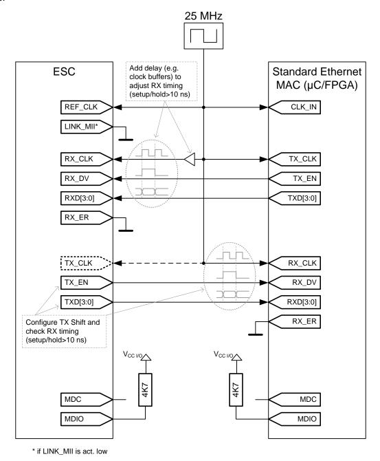
Figure 13: Back-to-Back MII Connection (ESC and standard MAC)
