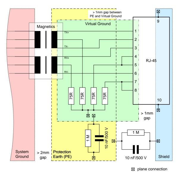
Figure 16: Termination and Grounding Recommendation
