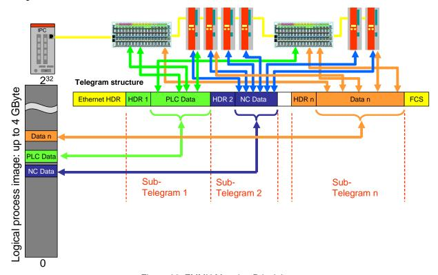
Figure 22: FMMU Mapping Principle
