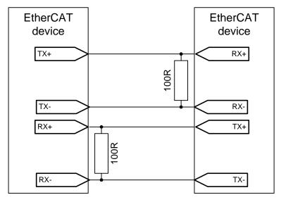
Figure 21: EBUS Connection
