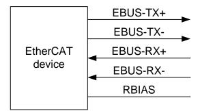
Figure 17: EBUS Interface Signals
