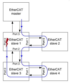
Figure 7: All frames are dropped because of Circulating Frame Prevention
