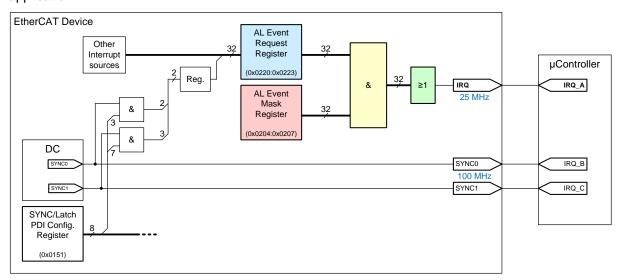
Figure 43: PDI Interrupt Masking and interrupt signals
