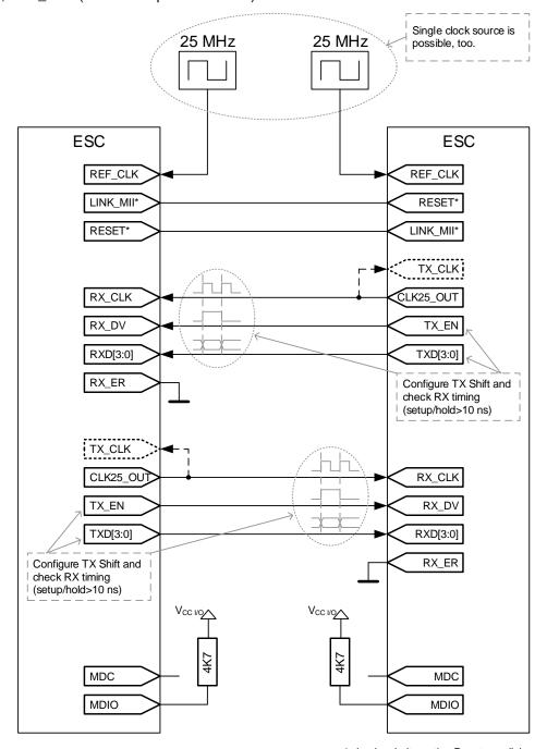
\* check polarity: active Reset = no link
