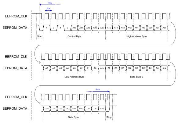
Figure 41: Write access (2 address bytes, 32 Kbit - 4 Mbit EEPROMs)
