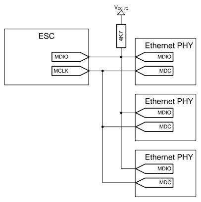
Figure 11: MII management example schematic
