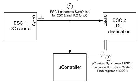
Figure 35: System Time PDI Controlled with two steps
