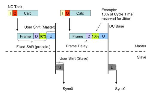
Figure 36: DC Timing Signals in relation to Communication
