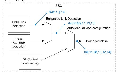
Figure 19: EBUS Link detection
