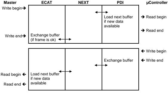
Figure 25: SyncManager Buffered Mode Interaction
