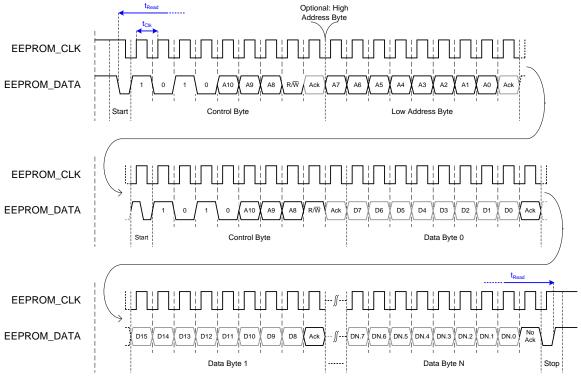
Figure 42: Read access (1 address byte, up to 16 Kbit EEPROMs)
