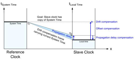
Figure 29: Propagation Delay, Offset, and Drift Compensation
