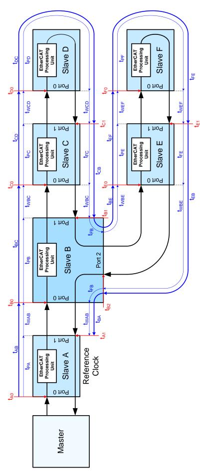
Figure 30: Propagation Delay Calculation
