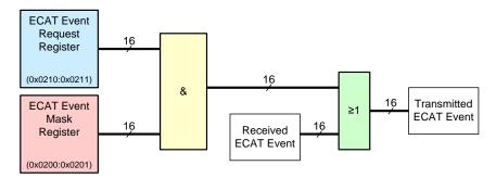
Figure 44: ECAT Interrupt Masking
