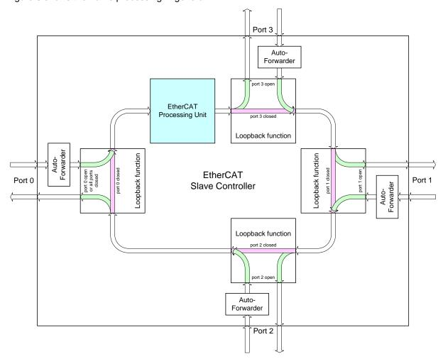
Figure 5: Frame Processing
