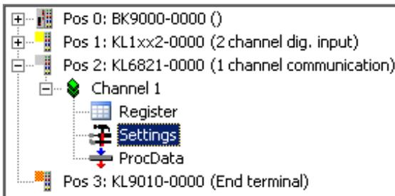
Fig. 15: KS2000 tree branches for channel 1 of the KL6821
