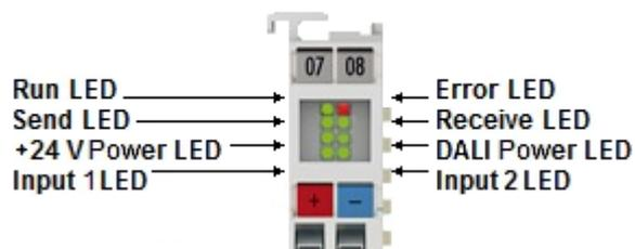
Fig. 12: KL6821 LEDs
