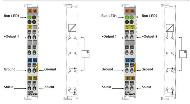
Fig. 11: KL4001, KL4002 - connection and LEDs
