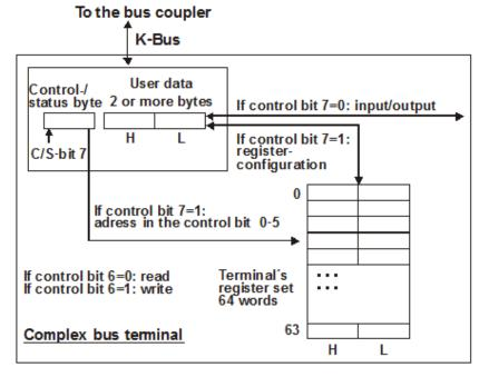
Fig. 17: Register mode control byte
