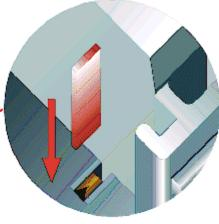
Fig. 6: Power contact on left side
