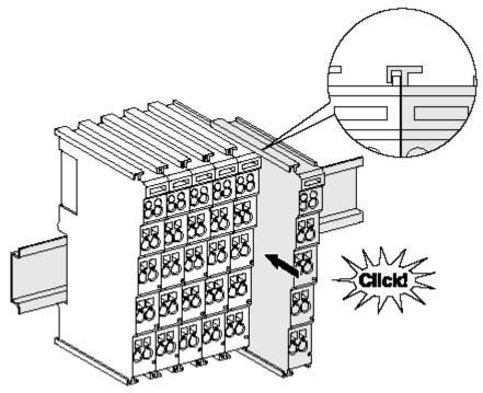
Fig. 4: Attaching on mounting rail
