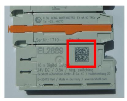
Fig. 1: BIC as data matrix code (DMC, code scheme ECC200)
