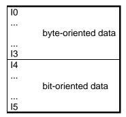
The base addresses I0 and O0 listed here are handled as relative addresses or addresses in the bus coupler. A base peripheral address can be assigned to the base address of the bus coupler in the bus master software. All following addresses are automatically assigned the successive addresses depending on the length of the actual data words.
