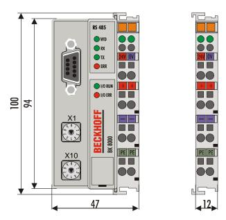
The overall width of the construction is the width of the bus coupler, including the bus end terminal, plus the width of the installed bus terminals. The bus terminals are 12 mm or 24 mm wide, depending on their function. Depending on the gauge of cables used the overall height of 68 mm may be overstepped by about 5 mm to 10 mm by the cables at the front.
