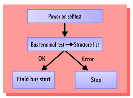
The bus coupler reports the error to the master by means of the Profibus diagnostics. Clearing the error returns the bus coupler to its normal operating mode.
