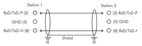
In systems with more than two stations all devices are wired in parallel. In order to be able to loop through the cable without interruption, two cables must be connected to one plug. 9-pin D-sub plugs with switchable terminal resistors, guaranteeing a straightforward cable connection, can be obtained from Beckhoff.
