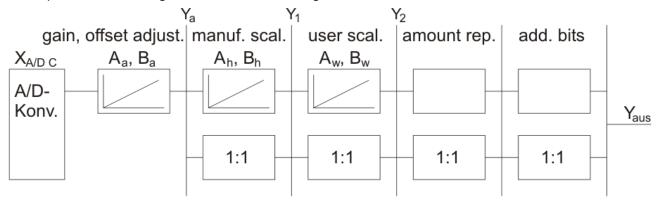
Fig. 6: Signal processing
