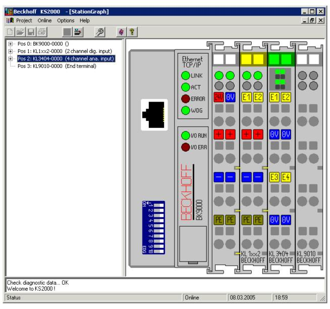
Fig. 18: Display of the fieldbus station in KS2000
