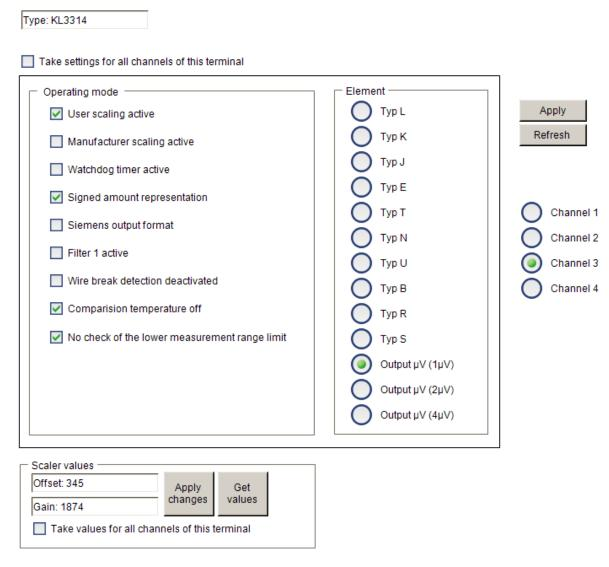
Fig. 22: Settings of KL3314 via visualization of TwinCAT 3
