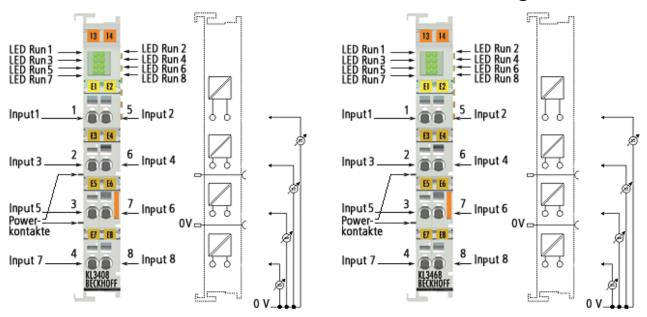
Fig. 16: KL3408 and KL3468 - Contact assignment
