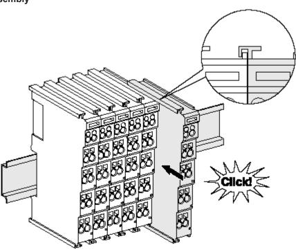
Fig. 8: Attaching on mounting rail
