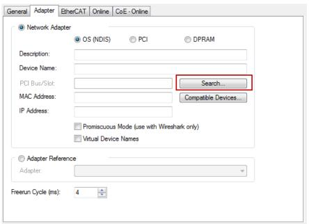
Fig. 24: Search of the existing HW configuration for the EtherCAT configuration of the example
