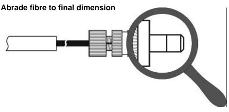
Do not cut off the protruding fibre end, because this could lead to crack formation, but
