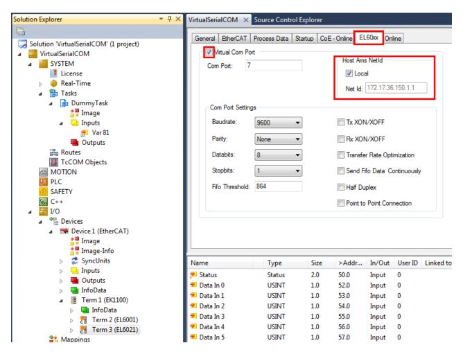
The EL6021 does not support RTS/CTS handshake. It does support a half duplex mode and it can be configured for point to point connections.
