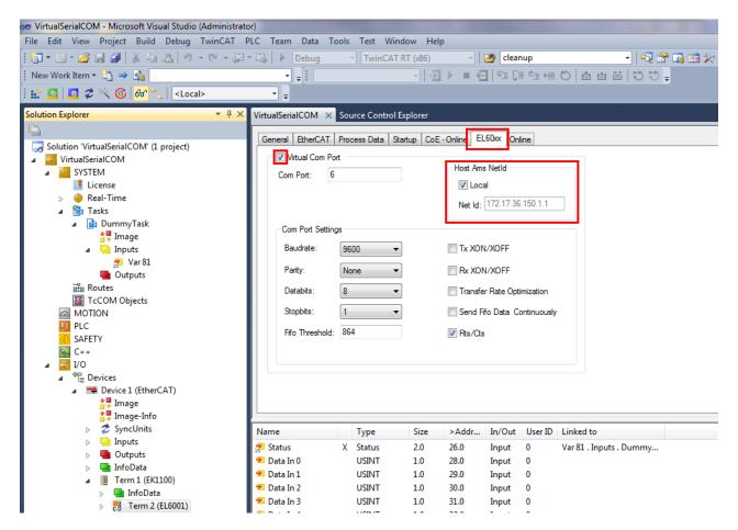
The number of the COM port is defined in edit field "Com Port". Note, that a com port number must be unique within a computer. The computer on which the virtual com port should be created must not have a com port with this number. TwinCAT starts with com port number 6. The com port number must be less than 65536.
