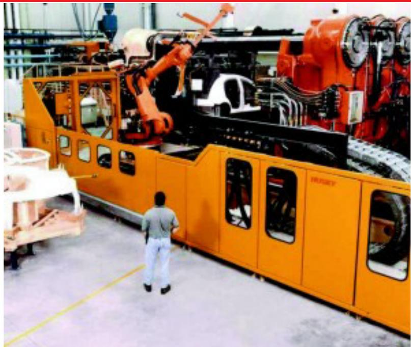
the material through the machine nozzle into the mold cavities, and to keep the melt under pressure. After a specific mold cooling time, the screw piston is pulled back. The mold is opened, and the molded parts are removed from the mold cores either by means of an ejection mechanism or by a robot. The machine cycle can then be resumed anew. Suitable machines for this process must meet a whole set of requirements, importantly:
