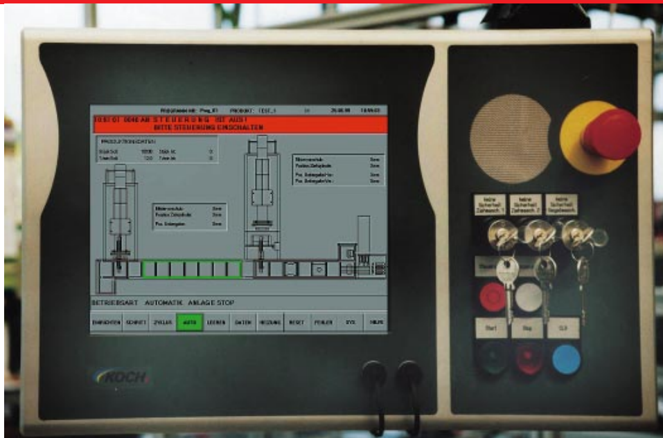
The Human Machine Interface is done with the Beckhoff Control Panel, which can be installed up to 65 m away from the control PC.
