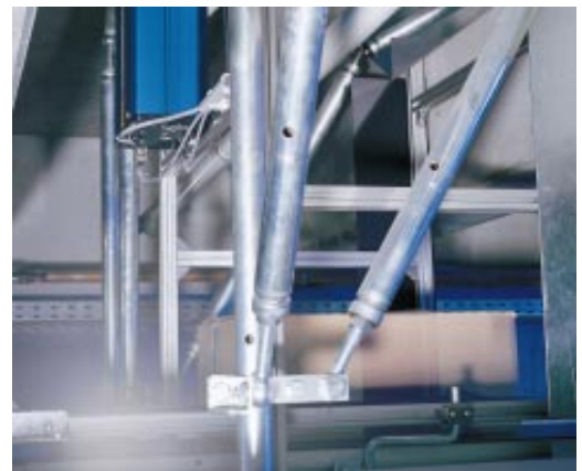
Scanners, communicating with the computer via the Lightbus, generate signals for the material flow.
