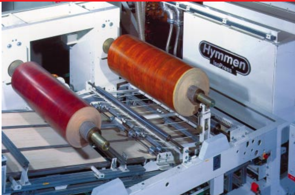
Several machines are chained up with each other in the wood processing installation of Hymmen. The various installation parts are controlled by the TwinCAT software that is based on Windows NT.
